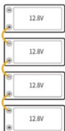
Series Connection 48V(51.2V) 200Ah
